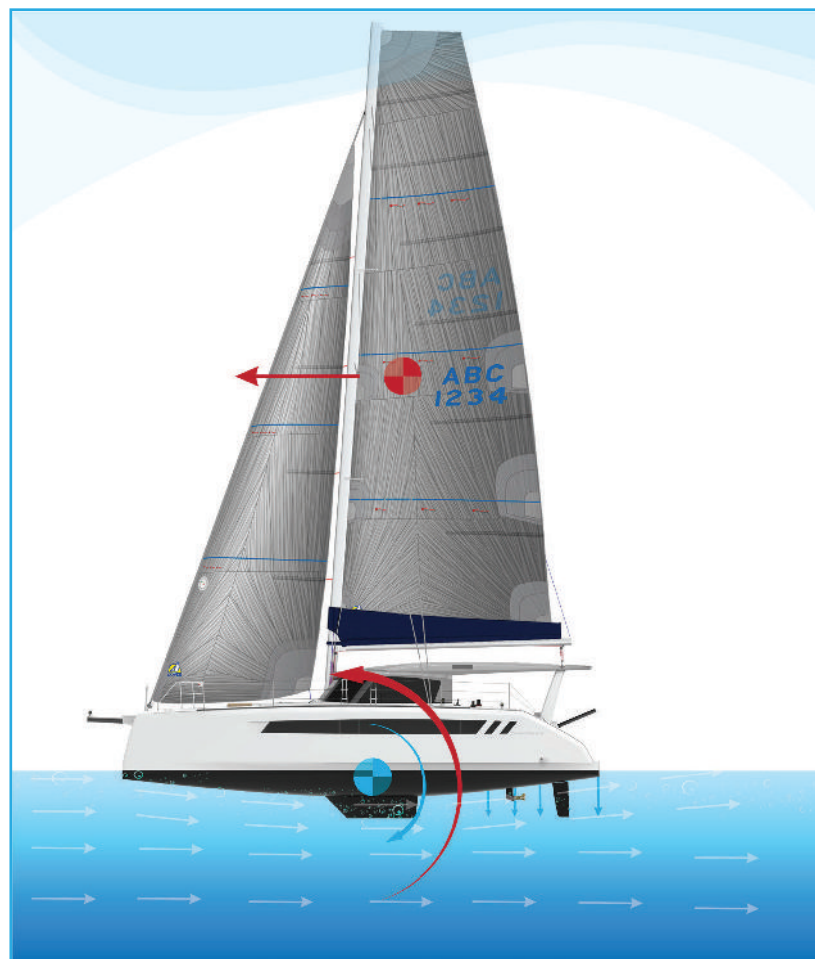
How the aft rocker counter affects the pitching moments thanks to Coandar effect.
