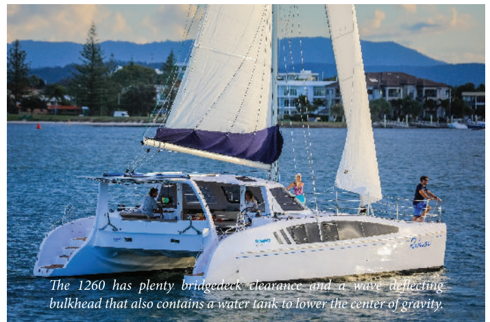
A simple sailplan of self-tacking jib and accessible mainsail makes the 1260 an ideal short-handed cruiser.
